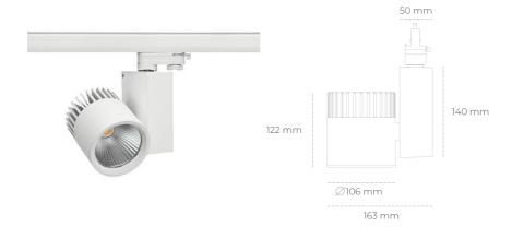
COB Light colour 2000 [K] MEAT PINK CRI Led chip flux 1845 [lm] Luminous flux 1476 [lm] System power 21 [W] Luminaire Efficiency 70 [lm/W] Beam angle 45° Controller ON/OFF MacAdam 3 SDCM
