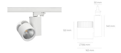
COB Light colour 4000 [K] | CRI 3866 [lm] Led chip flux Luminous flux 3092 [lm] System power 31 [W] Luminaire Efficiency 100 [lm/W] Beam angle 45° Controller ON/OFF MacAdam 3 SDCM
