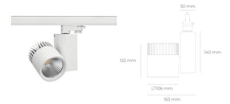
COB Light colour 4000 [K] | CRI Led chip flux 2416 [lm] Luminous flux 1932 [lm] System power 19 [W] Luminaire Efficiency 102 [lm/W] Beam angle 30° Controller ON/OFF MacAdam 3 SDCM
