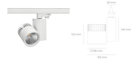
COB Light colour 4000 [K] | CRI Led chip flux 3141 [lm] Luminous flux 2512 [lm] System power 25 [W] Luminaire Efficiency 100 [lm/W] Beam angle 15° Controller ON/OFF MacAdam 3 SDCM
