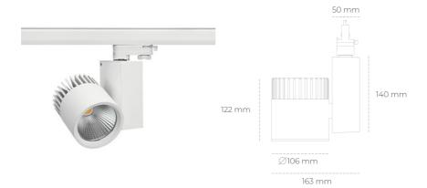
COB Light colour 2700 [K] | CRI Led chip flux 1111 [lm] Luminous flux 888 [lm] System power 10 [W] Luminaire Efficiency 89 [lm/W] Beam angle 60° Controller ON/OFF MacAdam 3 SDCM
