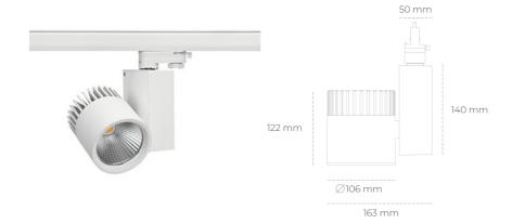
COB Light colour 2700 [K] | CRI 2888 [lm] Led chip flux Luminous flux 2310 [lm] System power 25 [W] Luminaire Efficiency 92 [lm/W] Beam angle 20° Controller ON/OFF MacAdam 3 SDCM
