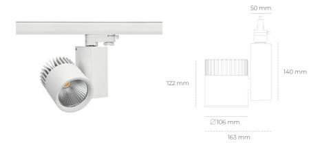
COB Light colour 5000 [K] | CRI Led chip flux 2895 [lm] Luminous flux 2316 [lm] System power 19 [W] Luminaire Efficiency 122 [lm/W] Beam angle 45° Controller ON/OFF MacAdam 3 SDCM
