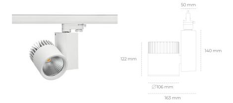
COB Light colour 5000 [K] | CRI Led chip flux 2027 [lm] Luminous flux 1621 [lm] System power 14 [W] Luminaire Efficiency 116 [lm/W] Beam angle 30° Controller ON/OFF MacAdam 3 SDCM
