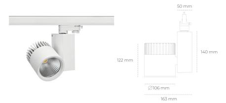
COB Light colour 5000 [K] | CRI Led chip flux 3475 [lm] Luminous flux 2780 [lm] System power 23 [W] Luminaire Efficiency 121 [lm/W] Beam angle 15° Controller ON/OFF MacAdam 3 SDCM
