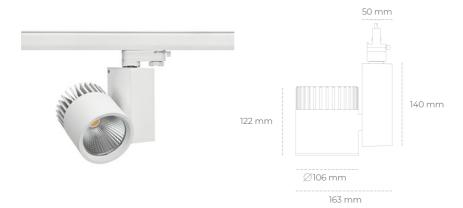
COB Light colour 3500 [K] | CRI Led chip flux 1391 [lm] Luminous flux 1112 [lm] System power 10 [W] Luminaire Efficiency 111 [lm/W] Beam angle 45° Controller ON/OFF MacAdam 3 SDCM
