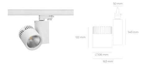
COB Light colour 3500 [K] | CRI Led chip flux 2783 [lm] Luminous flux 2226 [lm] System power 19 [W] Luminaire Efficiency 117 [lm/W] Beam angle 20° Controller ON/OFF MacAdam 3 SDCM
