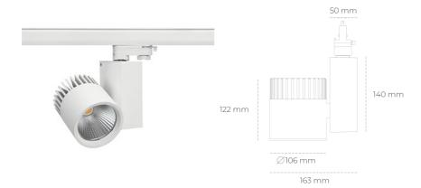
COB Light colour 3000 [K] | CRI 4900 [lm] Led chip flux Luminous flux 3920 [lm] System power 35 [W] Luminaire Efficiency 112 [lm/W] Beam angle 60° Controller ON/OFF MacAdam 3 SDCM
