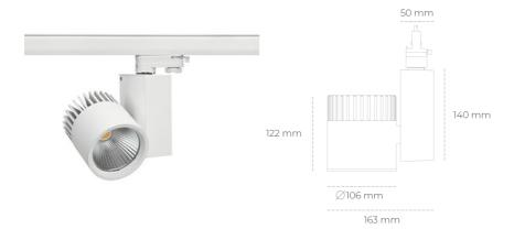
COB Light colour 3000 [K] | CRI Led chip flux 1361 [lm] Luminous flux 1088 [lm] System power 10 [W] Luminaire Efficiency 109 [lm/W] Beam angle 15° Controller ON/OFF MacAdam 3 SDCM
