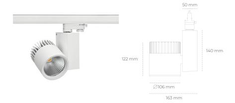
COB Light colour 2700 [K] | CRI Led chip flux 4850 [lm] Luminous flux 3880 [lm] System power 35 [W] Luminaire Efficiency 111 [lm/W] Beam angle 20° Controller ON/OFF MacAdam 3 SDCM
