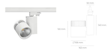
COB Light colour 2700 [K] | CRI Led chip flux 2694 [lm] Luminous flux 2155 [lm] System power 19 [W] Luminaire Efficiency 113 [lm/W] Beam angle 20° Controller ON/OFF MacAdam 3 SDCM
