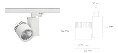
COB Light colour 2700 [K] | CRI Led chip flux 3772 [lm] Luminous flux 3017 [lm] System power 27 [W] Luminaire Efficiency 112 [lm/W] Beam angle 15° Controller ON/OFF MacAdam 3 SDCM
