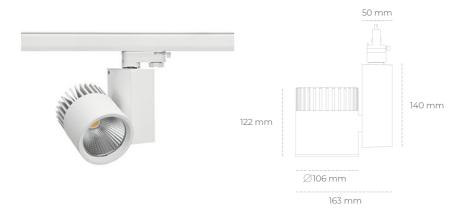
COB 4000 [K] PREMIUM WHITE Light colour CRI 90 Led chip flux 2663 [lm] Luminous flux 2130 [lm] System power 20 [W] Luminaire Efficiency 107 [lm/W] Beam angle 45° Controller ON/OFF MacAdam 3 SDCM
