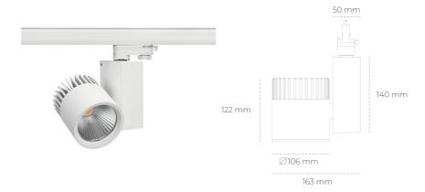
COB 4000 [K] PREMIUM WHITE Light colour CRI 90 Led chip flux 4545 [lm] Luminous flux 3636 [lm] System power 35 [W] Luminaire Efficiency 104 [lm/W] Beam angle 20° Controller ON/OFF MacAdam 3 SDCM
