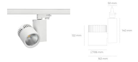
COB 4000 [K] PREMIUM WHITE Light colour CRI 90 Led chip flux 3398 [lm] Luminous flux 2718 [lm] System power 25 [W] Luminaire Efficiency 109 [lm/W] Beam angle 20° Controller ON/OFF MacAdam 3 SDCM
