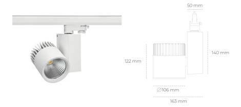
COB 4000 [K] PREMIUM WHITE Light colour CRI 90 Led chip flux 3398 [lm] Luminous flux 2718 [lm] System power 25 [W] Luminaire Efficiency 109 [lm/W] Beam angle 15° Controller ON/OFF MacAdam 3 SDCM
