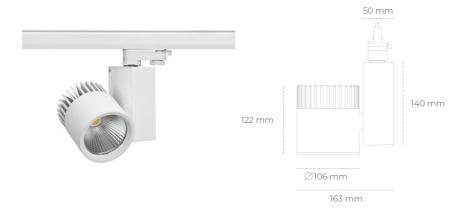
COB 3000 [K] PREMIUM COLOR Light colour CRI 90 Led chip flux 3317 [lm] Luminous flux 2653 [lm] System power 31 [W] Luminaire Efficiency 86 [lm/W] Beam angle 60° Controller ON/OFF MacAdam 3 SDCM
