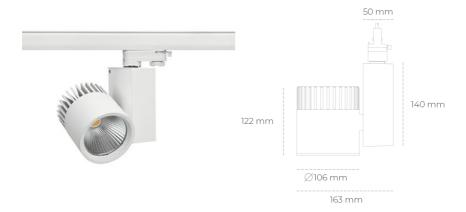
COB 3000 [K] PREMIUM COLOR Light colour CRI 90 Led chip flux 2960 [lm] Luminous flux 2368 [lm] System power 27 [W] Luminaire Efficiency 88 [lm/W] Beam angle 45° Controller ON/OFF MacAdam 3 SDCM
