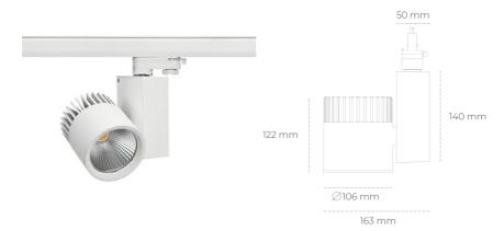
COB 3000 [K] PREMIUM COLOR Light colour CRI 90 Led chip flux 1145 [lm] Luminous flux 916 [lm] System power 11 [W] Luminaire Efficiency 83 [lm/W] Beam angle 45° Controller ON/OFF MacAdam 3 SDCM
