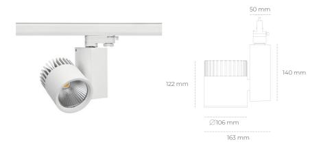
COB 3000 [K] PREMIUM COLOR Light colour CRI 90 Led chip flux 3317 [lm] Luminous flux 2653 [lm] System power 31 [W] Luminaire Efficiency 86 [lm/W] Beam angle 20° Controller ON/OFF MacAdam 3 SDCM
