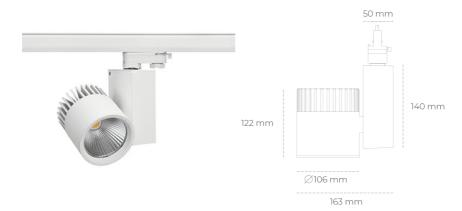
COB 3000 [K] PREMIUM COLOR Light colour CRI 90 Led chip flux 2776 [lm] Luminous flux 2220 [lm] System power 25 [W] Luminaire Efficiency 89 [lm/W] Beam angle 20° Controller ON/OFF MacAdam 3 SDCM
