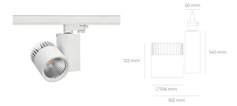
COB 3000 [K] PREMIUM COLOR Light colour CRI 90 Led chip flux 3827 [lm] Luminous flux 3061 [lm] System power 37 [W] Luminaire Efficiency 83 [lm/W] Beam angle 15° Controller ON/OFF MacAdam 3 SDCM
