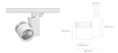
COB 3000 [K] CRI97 Light colour CRI Led chip flux 2990 [lm] Luminous flux 2392 [lm] System power 27 [W] Luminaire Efficiency 89 [lm/W] Beam angle 45° Controller ON/OFF MacAdam 3 SDCM
