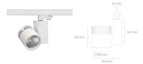
COB 3000 [K] CRI97 Light colour CRI 2199 [lm] Led chip flux Luminous flux 1759 [lm] System power 19 [W] Luminaire Efficiency 93 [lm/W] Beam angle 45° Controller ON/OFF MacAdam 3 SDCM
