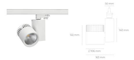
COB 3000 [K] CRI97 Light colour CRI Led chip flux 1575 [lm] Luminous flux 1260 [lm] System power 14 [W] Luminaire Efficiency 90 [lm/W] Beam angle 45° Controller ON/OFF MacAdam 3 SDCM
