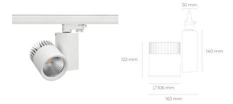
COB 3000 [K] CRI97 Light colour CRI Led chip flux 1575 [lm] Luminous flux 1260 [lm] System power 14 [W] Luminaire Efficiency 90 [lm/W] Beam angle 30° Controller ON/OFF MacAdam 3 SDCM
