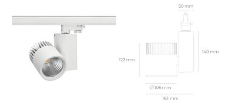
COB 3000 [K] PREMIUM WHITE Light colour CRI 90 Led chip flux 3911 [lm] Luminous flux 3128 [lm] System power 27 [W] Luminaire Efficiency 116 [lm/W] Beam angle 45° Controller
