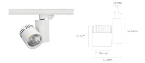
COB Light colour 5700 [K] SPECIAL CRI 3023 [lm] Led chip flux Luminous flux 2418 [lm] System power 23 [W] Luminaire Efficiency 105 [lm/W] Beam angle 30° Controller ON/OFF MacAdam 3 SDCM
