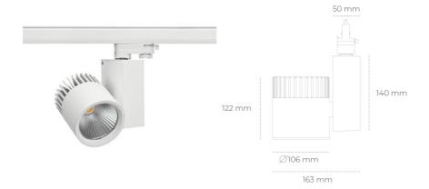
COB Light colour 5700 [K] SPECIAL CRI Led chip flux 2788 [lm] Luminous flux 2230 [lm] System power 21 [W] Luminaire Efficiency 106 [lm/W] Beam angle 30° Controller ON/OFF MacAdam 3 SDCM
