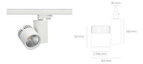
COB Light colour 5700 [K] SPECIAL CRI 3484 [lm] Led chip flux Luminous flux 2787 [lm] System power 27 [W] Luminaire Efficiency 103 [lm/W] Beam angle 20° Controller ON/OFF MacAdam 3 SDCM
