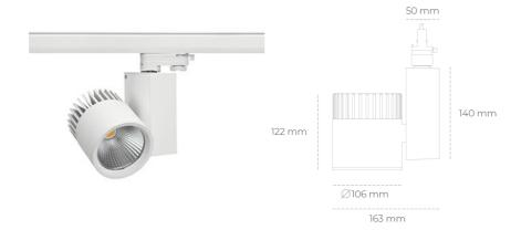
COB Light colour 5700 [K] SPECIAL CRI 3023 [lm] Led chip flux Luminous flux 2418 [lm] System power 23 [W] Luminaire Efficiency 105 [lm/W] Beam angle 20° Controller ON/OFF MacAdam 3 SDCM
