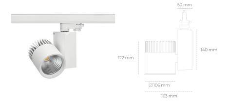
COB 4200 [K] MEAT WHITE Light colour CRI 90 Led chip flux 3539 [lm] Luminous flux 2831 [lm] System power 37 [W] Luminaire Efficiency 77 [Im/W] Beam angle 45° Controller ON/OFF MacAdam 3 SDCM
