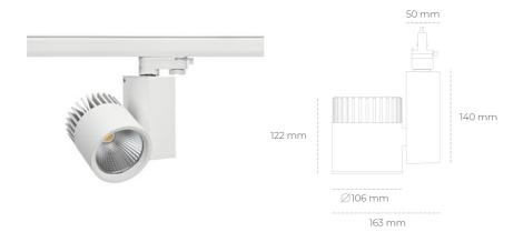
COB 4200 [K] MEAT WHITE Light colour CRI 90 Led chip flux 2695 [lm] Luminous flux 2156 [lm] System power 27 [W] Luminaire Efficiency 80 [lm/W] Beam angle 45° Controller ON/OFF MacAdam 3 SDCM
