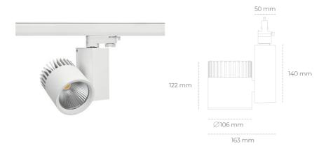
COB 4000 [K] HI EFFICIENT Light colour CRI 90 Led chip flux 3793 [lm] Luminous flux 3034 [lm] System power 23 [W] Luminaire Efficiency 132 [lm/W] Beam angle 60° Controller ON/OFF MacAdam 3 SDCM
