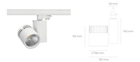
COB 4000 [K] HI EFFICIENT Light colour CRI 90 Led chip flux 5532 [lm] Luminous flux 4425 [lm] System power 34 [W] Luminaire Efficiency 130 [lm/W] Beam angle 45° Controller ON/OFF MacAdam 3 SDCM
