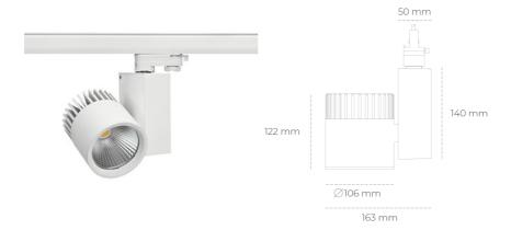
COB 4000 [K] HI EFFICIENT Light colour CRI 90 Led chip flux 3793 [lm] Luminous flux 3034 [lm] System power 23 [W] Luminaire Efficiency 132 [lm/W] Beam angle 20° Controller ON/OFF MacAdam 3 SDCM
