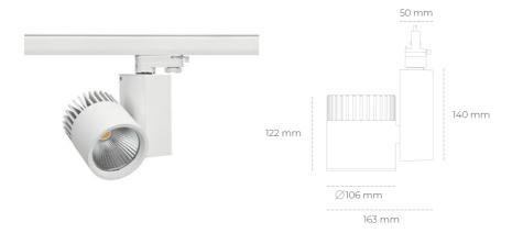
COB 4000 [K] HI EFFICIENT Light colour CRI 90 Led chip flux 3189 [lm] Luminous flux 2551 [lm] System power 19 [W] Luminaire Efficiency 134 [lm/W] Beam angle 20° Controller ON/OFF MacAdam 3 SDCM
