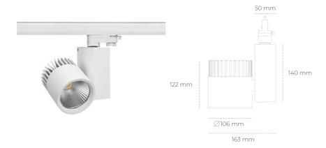
COB 4000 [K] HI EFFICIENT Light colour CRI 90 Led chip flux 2260 [lm] Luminous flux 1808 [lm] System power 14 [W] Luminaire Efficiency 129 [lm/W] Beam angle 20° Controller ON/OFF MacAdam 3 SDCM
