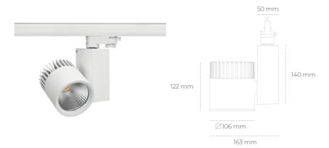
COB 3500 [K] HI EFFICIENT Light colour CRI 90 Led chip flux 1571 [lm] Luminous flux 1256 [lm] System power 10 [W] Luminaire Efficiency 126 [lm/W] Beam angle 60° Controller ON/OFF MacAdam 3 SDCM
