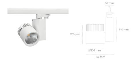
COB 3500 [K] HI EFFICIENT Light colour CRI 90 Led chip flux 3904 [lm] Luminous flux 3123 [lm] System power 25 [W] Luminaire Efficiency 125 [lm/W] Beam angle 45° Controller ON/OFF MacAdam 3 SDCM
