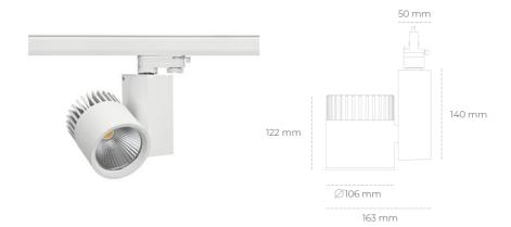
COB 3500 [K] HI EFFICIENT Light colour CRI 90 Led chip flux 1571 [lm] Luminous flux 1256 [lm] System power 10 [W] Luminaire Efficiency 126 [lm/W] Beam angle 45° Controller ON/OFF MacAdam 3 SDCM
