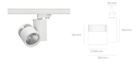
COB 3500 [K] HI EFFICIENT Light colour CRI 90 Led chip flux 3904 [lm] Luminous flux 3123 [lm] System power 25 [W] Luminaire Efficiency 125 [lm/W] Beam angle 30° Controller ON/OFF MacAdam 3 SDCM
