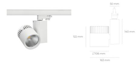
COB 3000 [K] HI EFFICIENT Light colour CRI 90 Led chip flux 4378 [lm] Luminous flux 3502 [lm] System power 27 [W] Luminaire Efficiency 130 [lm/W] Beam angle 30° Controller ON/OFF MacAdam 3 SDCM
