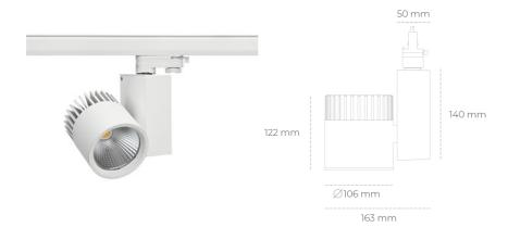
COB 3000 [K] HI EFFICIENT Light colour CRI 90 Led chip flux 2256 [lm] Luminous flux 1804 [lm] System power 14 [W] Luminaire Efficiency 129 [lm/W] Beam angle 30° Controller ON/OFF MacAdam 3 SDCM
