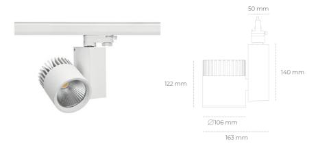
COB 3000 [K] HI EFFICIENT Light colour CRI 90 Led chip flux 4378 [lm] Luminous flux 3502 [lm] System power 27 [W] Luminaire Efficiency 130 [lm/W] Beam angle 15° Controller ON/OFF MacAdam 3 SDCM
