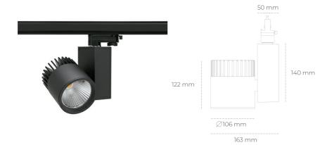
COB 2500 [K] BREAD Light colour CRI 2574 [lm] Led chip flux Luminous flux 2059 [lm] System power 21 [W] Luminaire Efficiency 98 [lm/W] Beam angle 20° Controller ON/OFF MacAdam 3 SDCM
